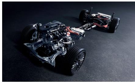
2.5L DYNAMIC FORCE ENGINE A25A-FXS × MOTOR・2WD/4WD
